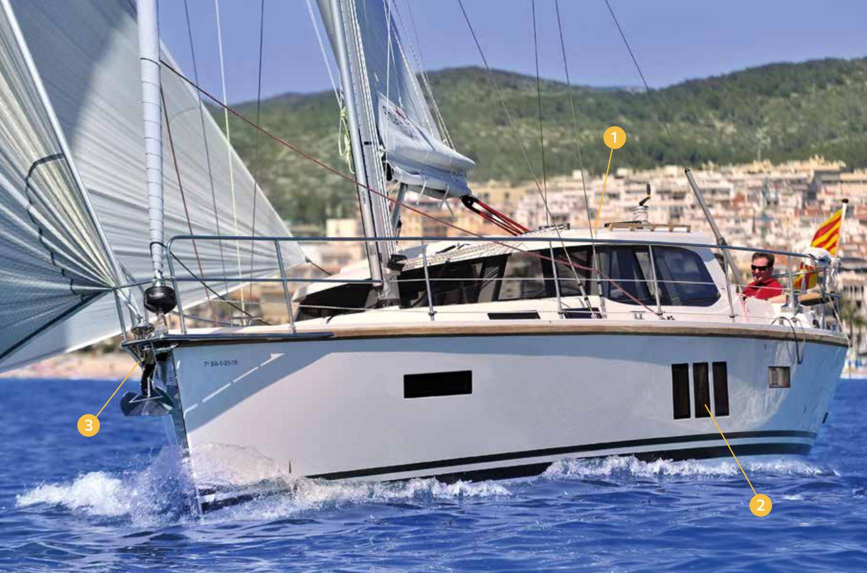
the helmsman, being hooked on to a stanchion that is also an integral part of the cockpit table. The mainsheet is on an 8:1 system and is secured with a Harken camcleat. There are two large Andersen winches set well aft and also within easy reach of the helmsman and a single electric winch on the deckhouse used for raising and lowering sails.
