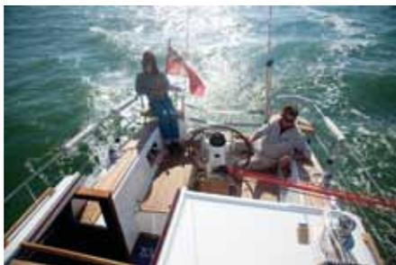
**Whether steering is by wheel or the standard tiller, sheets are within easy reach and the ergonomics of the deep cockpit are good**
